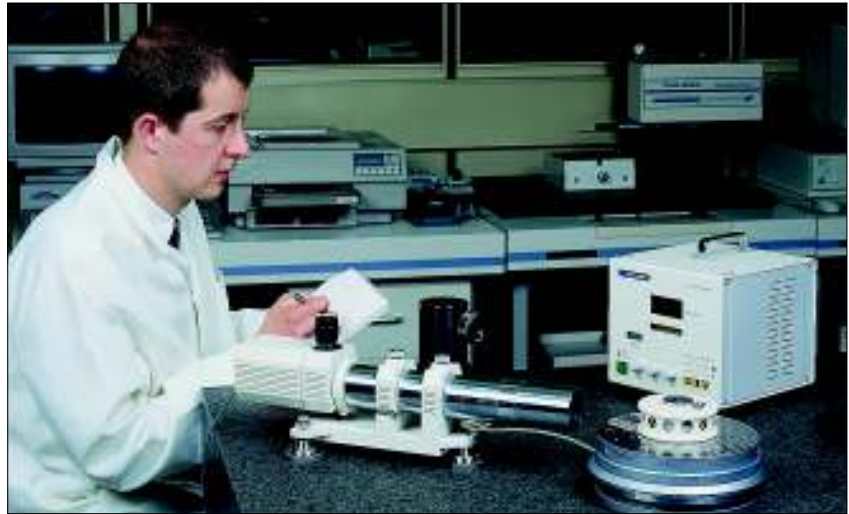
DA20 Autocollimator with reference index table used to calibrate a polygon
