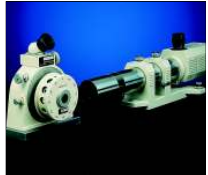
Checking a TB100 Clinometer with the TA51 Autocollimator
