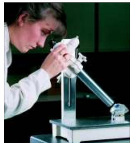
The VA900 Microptic Dual Axis Autocollimator
