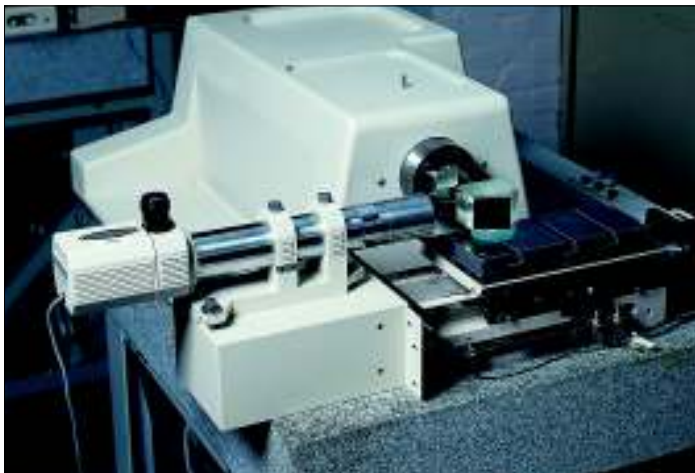
Precision Machine Tool alignment using DA20 Autocollimator
